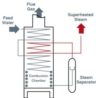
**Power Stations** have benefited by using the Clayton Steam Generator where superheated steam, high pressure steam and rapid start capability combined with the inherent safety have particular benefits. In both conventional and nuclear power stations the Clayton Steam Generator is used for peak shaving, auxiliary start-up steam, back-up steam supply and emergency steam.
