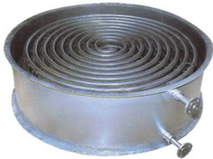
Because of the modular construction of the Clayton Exhaust Gas Boiler the assembly is a straightforward matter since the standard coil sections are bolted together and coned transition pieces are then added onto each end for connecting to the exhaust ducting. The water connections between each section are made on the outside of the boiler shell and an effective sootblowing system is built into every Clayton Exhaust Gas Boiler.
