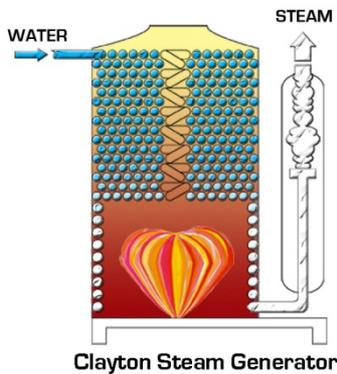
This is possible by pumping water through the inside of a small diameter heated coiled tube so that cold water goes in one end and high pressure steam comes out the other. The Clayton Steam Generator is a unique design that does just that. Instead of the familiar steam train image of a boiler we now have a compact steam making machine with staggering advantages for the world we live in today.
