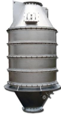
The Clayton Exhaust Gas Boiler can produce steam using the heat in the waste gases from diesel engines, small gas turbines, incinerators, glass furnaces, enamel ovens, stress relieving ovens and other suitable applications.
